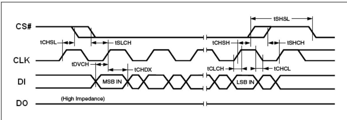
**Figure 24. Input Timing**
