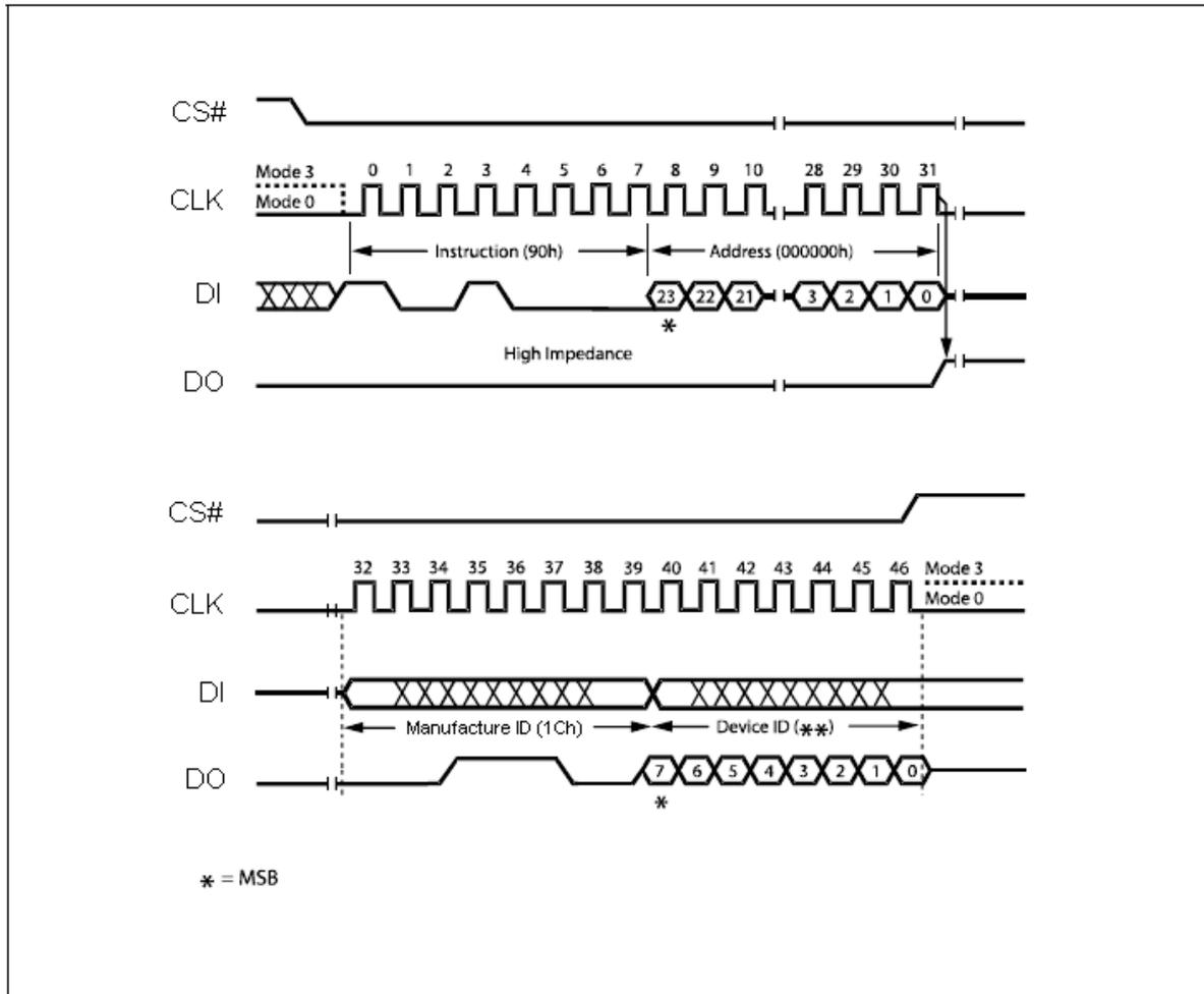
**Figure 18. Read Manufacturer / Device ID Diagram**
