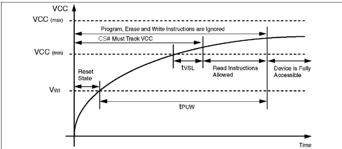
**Figure 21. Power-up Timing**
