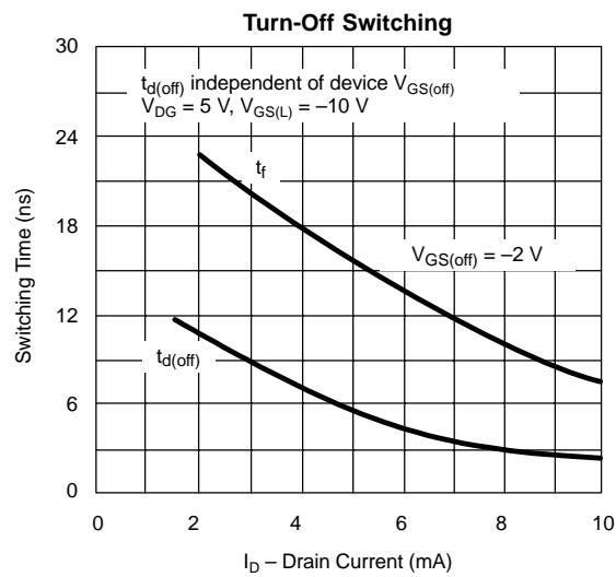
**TYPICAL CHARACTERISTICS ( $T_A = 25^\circ\text{C}$  UNLESS OTHERWISE NOTED)**
