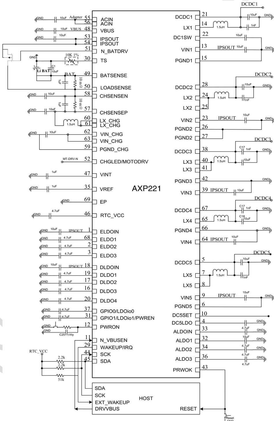
29/44/45 pin are pulled high to RTC\_VCC; 10 PIN IF is connected to VINT; DCDC5 outputs 1.35V; 10 PIN IF is connected to GND; DCDC5 outputs 1.5V; 10 PIN is floating; DCDC5 outputs 1.2V;
