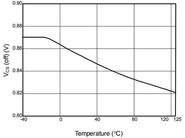
Fig. 8 V<sub>CS</sub> (off) vs. Temperature
