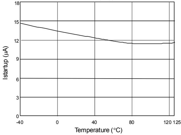
Fig. 9 Startup Current (I<sub>startup</sub>) vs. Temperature
