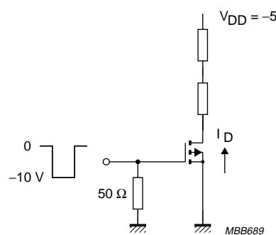
Fig.2 Switching times test circuit.
