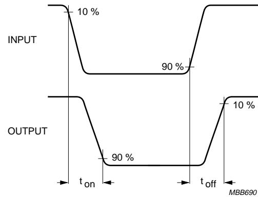
Fig.3 Input and output waveforms.
