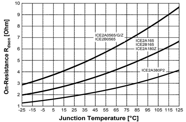
Figure 53 Drain Source On-Resistance  $R_{Dson}$  vs.  $T_j$
