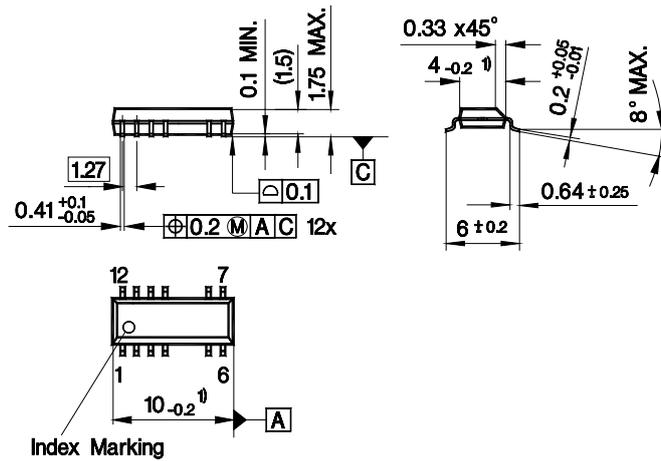
1) Does not include plastic or metal protrusion of 0.25 max. per side
