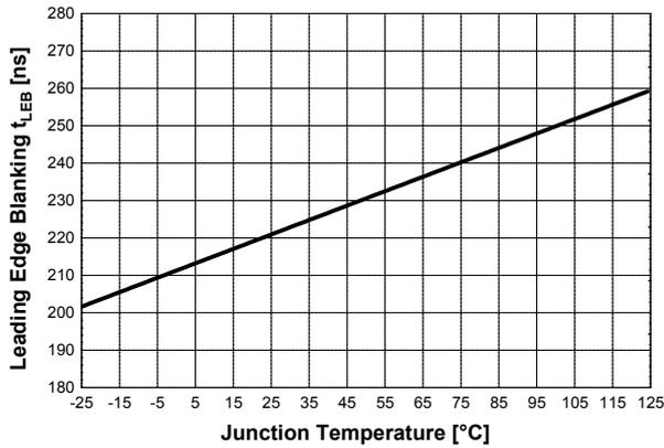
Figure 50 Leading Edge Blanking  $V_{VCC1}$  vs.  $T_j$
