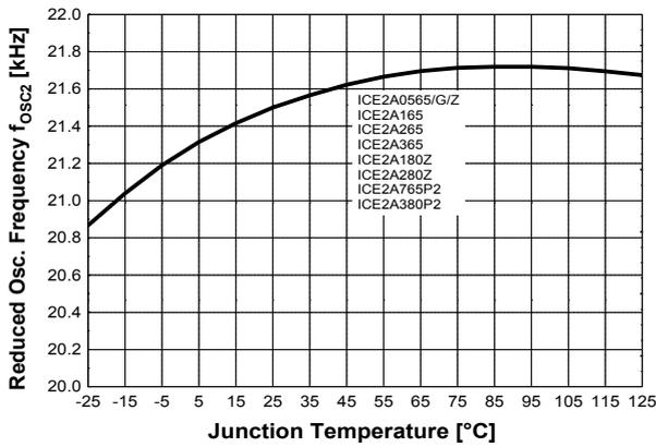
Figure 37 Reduced Osc. Frequency  $f_{OSC2}$  vs.  $T_j$
