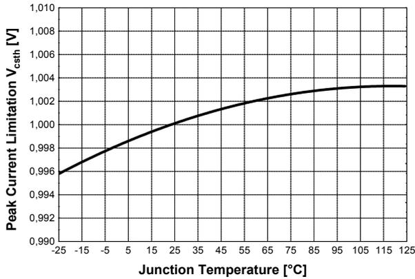
Figure 49 Peak Current Limitation  $V_{csth}$  vs.  $T_j$
