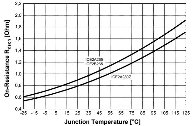
Figure 52 Drain Source On-Resistance  $R_{Dson}$  vs.  $T_j$
