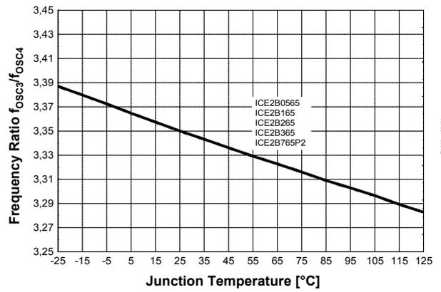
Figure 40 Frequency Ratio  $f_{OSC3} / f_{OSC4}$  vs.  $T_j$
