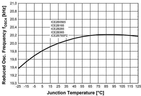
Figure 38 Reduced Osc. Frequency  $f_{OSC4}$  vs.  $T_j$
