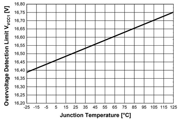
Figure 48 Overvoltage Detection Limit  $V_{VCC1}$  vs.  $T_j$
