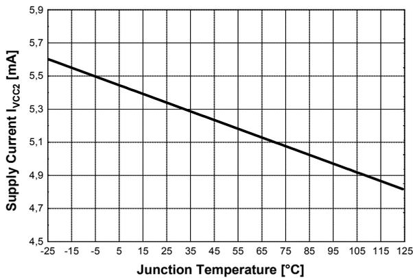
Figure 26 Static Supply Current  $I_{VCC2}$  vs.  $T_j$
