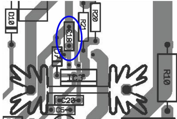
Figure 57B Detail X, Soft Start Capacitor C<sub>18</sub> Layout Recommendation
