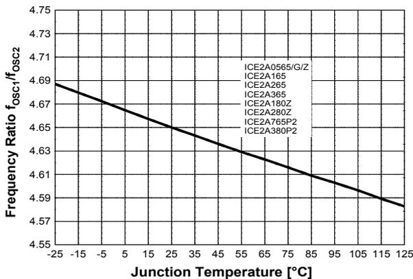
Figure 39 Frequency Ratio  $f_{OSC1} / f_{OSC2}$  vs.  $T_j$
