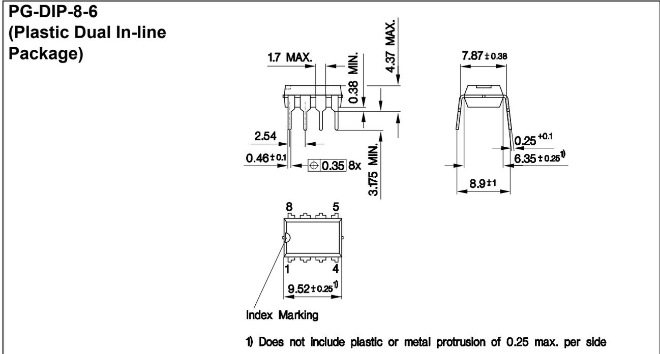
Figure 58 PG-DIP-8-6 (Plastic Dual In-line Package)
