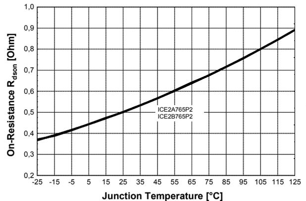
Figure 54 Drain Source On-Resistance  $R_{Dson}$  vs.  $T_j$
