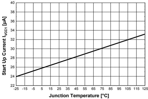
Figure 25 Start Up Current  $I_{VCC1}$  vs.  $T_j$
