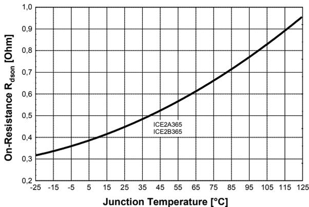
Figure 51 Drain Source On-Resistance  $R_{Dson}$  vs.  $T_j$
