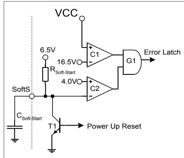
Figure 24 Overvoltage Detection
